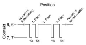
For versions with an impulse switch control, the output switches for 40 seconds at the beginning of each stage (terminal 7 or 7').
