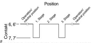
changes after each regeneration stage. With an odd number of the mechanical positions, operating position reset has to occur via the synchronous contact (operating switch). as impulse
